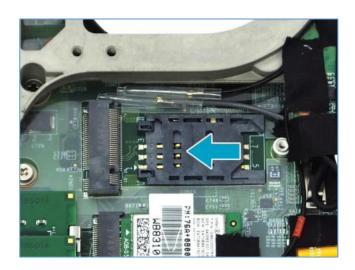
4. Lift the SIM card slot upwards.
