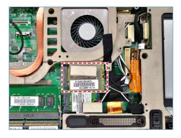
3. Push the SIM card slot forward to release it from the latch.
