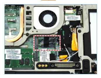
❖ With LTE module: Remove the screw securing the LTE module. Then carefully pull to disconnect the LTE module from the mainboard connector.
